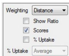
**Weighting** - This option determines how the polar maps are constructed. Distance weighting ensures that defect location is most accurate, while volume weighting ensures that defect size is most accurate. For more information, see manual section 8.2 (Polar Maps / SSS Options).
